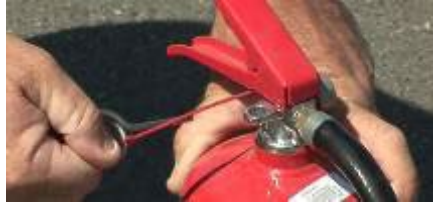
P – Pull out the safety pin
